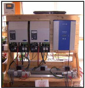
Figure 4: Test bench with Kaco Powador
