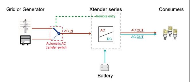
(Figure 1) Automatic management of two different energy sources
