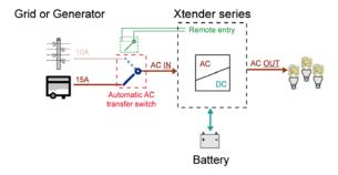
(Figure 5) System on generator connected
