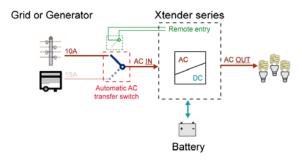
(Figure 3) System on grid connected
