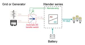
(Figure 4), System in mode "stand-alone"
