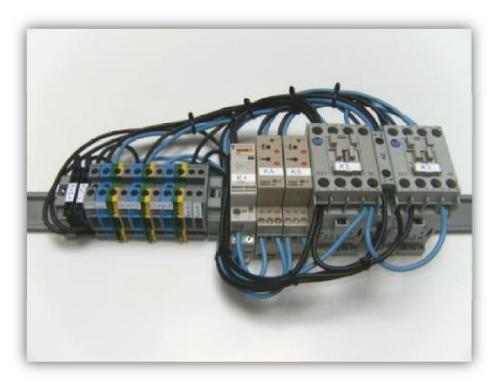
(Figure 11), Automatic AC transfer switch (wired)
