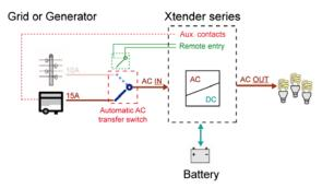
(Figure 8) System with an automatic generator startup
