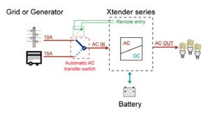
(Figure 6) System simultaneously connected the grid and on a generator
