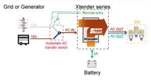
(Figure 7), System with the Smart-Boost function activated
