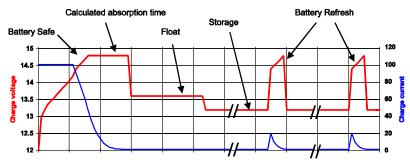
Fig. 4: Four-step adaptive charge curve
