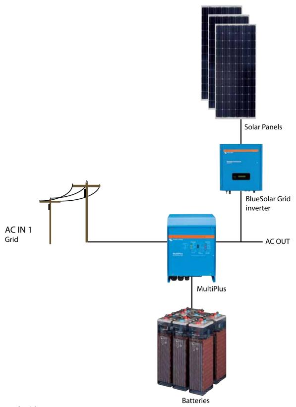
**2. Solar and grid**In this back-up system, AC from the grid can supplement the energy supply coming from the solar panels. And vice versa, the energy from the solar panels can cover any grid failure that may occur.
