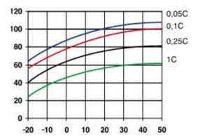
Fig. 1: Effect of temperature on capacity
