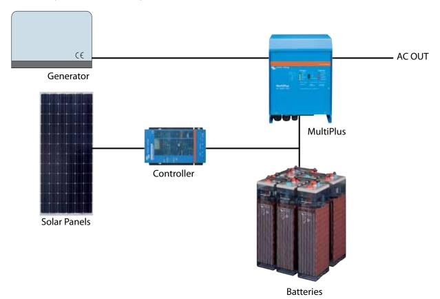
**3. Not enough sun – hybrid power** If the sun isn't providing you with enough energy, a generator is added to the system. In this case a Multiplus inverter/charger is used instead of an inverter. The generator is connected directly to the MultiPlus. The MultiPlus automatically regulates the starting and stopping of the generator, while maximizing the use of solar power and securing a long battery life.
