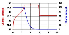
Fig. 3: Three step charge curve
