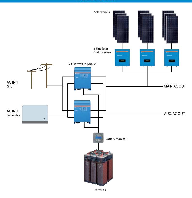
**2. AC system**The illustration above shows an AC system with three grid inverters and two Quattro's in parallel.
