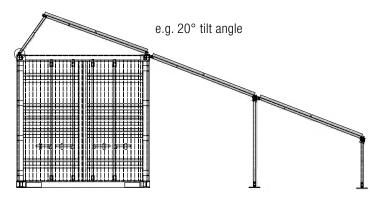
Storage Container incl. PV modules and modular mounting system
