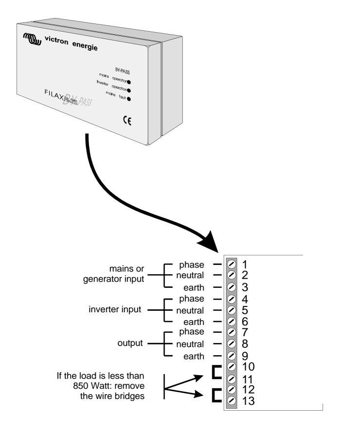
Figure 1. Connection diagram Filax
