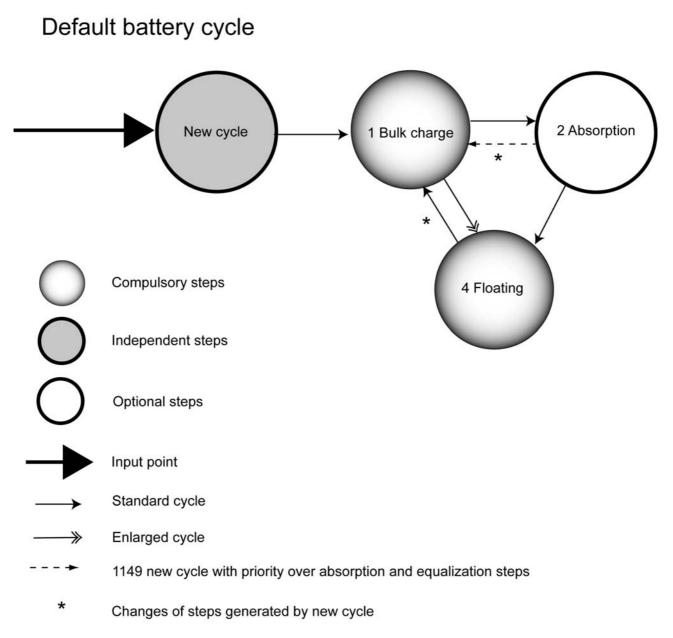
The battery cycle fits a large number of batteries by default, irrespective of whether they are gel batteries or not.
