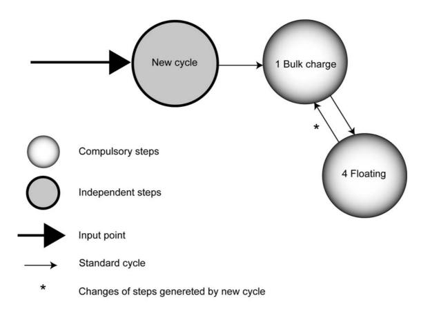
The bulk charge and floating phases cannot be deactivated. If the conditions for starting a new battery charge cycle have come together, the bulk charge phase starts immediately.
