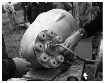
Fig. 4 Placing vibration isolators
