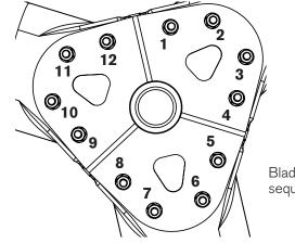
Blade bolt tightening sequence
