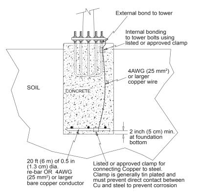
Fig. 4 Concrete encased electrode.
