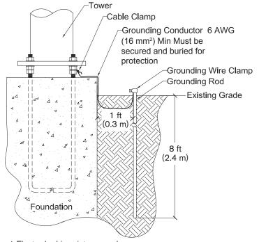
Fig. 1 Electrode driven into ground.
