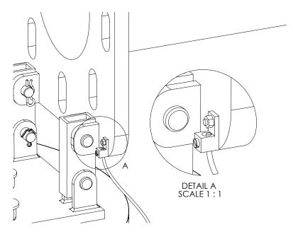
Fig. 2 Attaching the grounding wire to the tower base.
