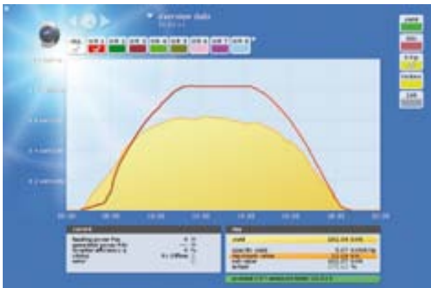
Inverter power restriction resulting from overheating or incorrect configuration
