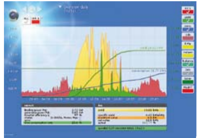
Daily summary with presentation of yield and power consumption balance, 1 inverter drawing down power (red), power generation (yellow), self-produced power (green)
