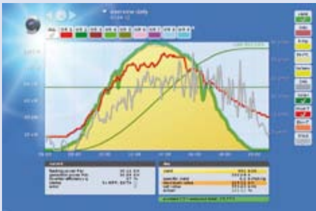
Daily curve with irradiance sensor (green), wind sensor (grey), module temperature (red) and yield curve (yellow)
