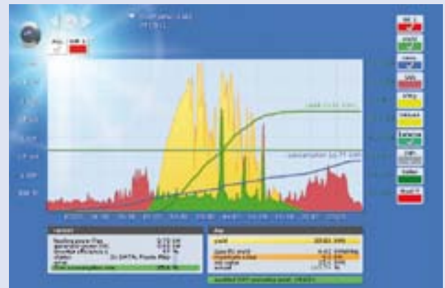
Daily overview with presentation of yield and consumption balance, 1 inverter current source (red), current production (yellow), "own current" (green)
