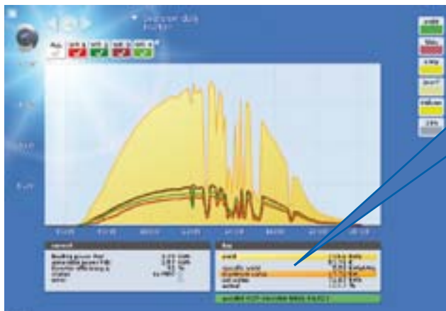
Daily overview with 4 inverters and shadowing
