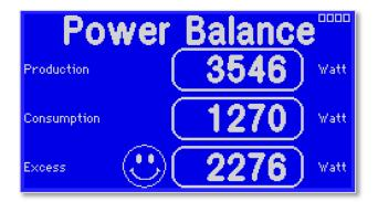
If a meter reader in the Solar-Log<sup>1000</sup> is configured with the "consumption meter" model, an additional "Power balance" dialogue box is available on the touchscreen. In this dialogue box, the current power values are shown and the surplus power is calculated. Depending on the surplus amount, a "smiley" indicates whether it makes sense or not to switch on consumers manually at that moment.
