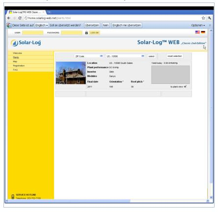
The overview shows the installed inverters, their output, module manufacturer, year of manufacture, orientation and the roof slope of the plants. If no picture of the plant has been made visible to all, a standard image is shown.
