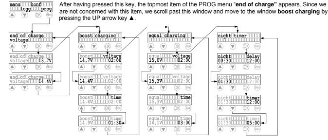
Once we reach the desired item "equal charging", then press the **OK** key to activate the window.
