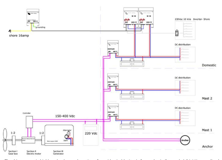
The drive system is highly redundant and consists of two identical "strings' of a mechanically coupled (bio) Yanmar diesel engine (55kW), a 20kW electrical motor/generator, a gearbox and a 'camber-adaptive' propeller.
