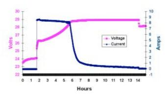
Example of a battery charge curve recorded with a BMV 602 and VEBat software
