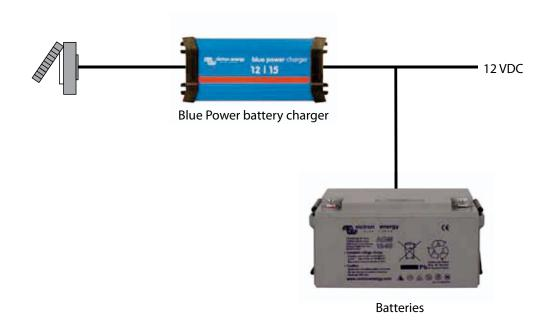
**1. Simple system with only DC consumers**The battery charger charges the battery and functions as a power supply for the consumers.
