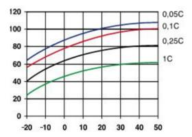
Fig. 1: Effect of temperature on capacity
