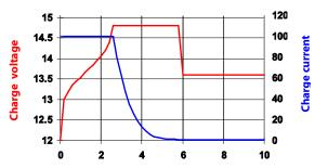
Fig. 3: Three step charge curve
