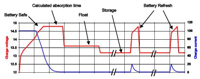
Fig. 4: Four-step adaptive charge curve
