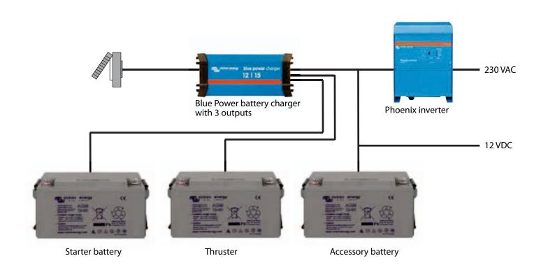
**2. System with inverter**This system contains an inverter to ensure a supply of 230VAC at all times. Many chargers have several outputs which allow for several battery groups to be charged separately.
