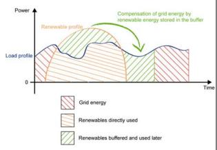
(Figure 4) Load profile with renewable energy buffered
