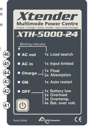
(42) This indicator lights up when the equipment has been stopped manually using the ON/OFF button (41). It also allows the cause of an unintentional stoppage of the device to be indicated via the different flashes, the imminence of a stoppage or the temporary limitation of its performance. The table below describes the type of fault according to the number of flashes on the indicator (42)
