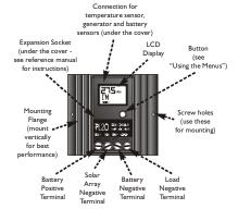
Screw wires into these terminals tightly.
