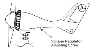
You can set the Wind Generator's stop charging point by the voltage regulator shown above.
