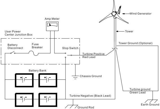
Higher input voltages from additional Wind Generators, solar panels, fuel-powered generators etc., can trick the Wind Generator's controller into sensing the battery in full charge, and the controller will prematurely stop charging. It will not harm the Wind Generator, just cause to slow down or stop spin. Please disconnect the other charging sources to determine the possible interference source.
