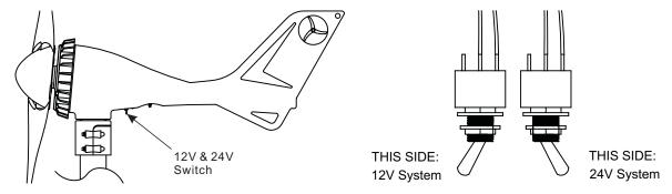
Would you want to change the output voltage? This is very easy, just change the position of the switch on the bottom of body. The 12V system is fit for lower wind speed and the 24V system is fit for higher wind speed. So, if you know your average wind speed is lower, please set the voltage to 12V. If the average wind speed is higher, please set the voltage to 24V.
