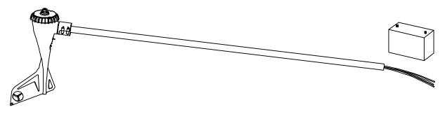
**6**/ Move the yaw shaft back up 1/8th inch (2mm) to prevent the bottom of the yaw from contacting the top of the pole. The only contact between the tower and yaw is through the rubber pad which will reduce the transmission of noise down the tower. Once the yaw shaft is on the tower, firmly tighten the yaw clamp screws with the 4mm hex key to 3-5 foot pounds (4.0-6.5Nm). Be sure that it is securely attached to the mounts.
