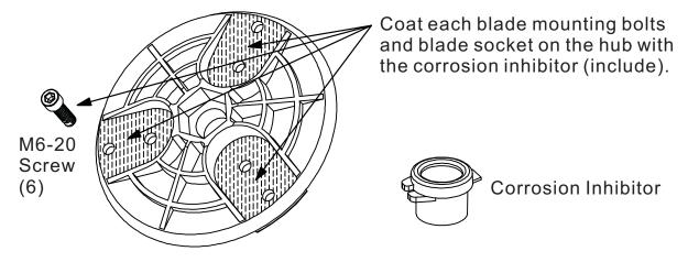
**9**/ Place one of the blades on the hub socket and insert one of the M6-20 socket head cap screws. Place a self-locking nut (M6) on the end of the screw and tighten it with the 5mm hex key to 8-10 foot lbs. (10.5-13.5 Nm). Repeat this procedure on all three blades.
