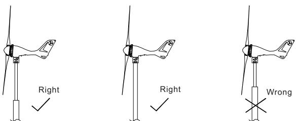
NOTE: No more than 8 feet (2.5m) of pipe should extend from the upper most support.
