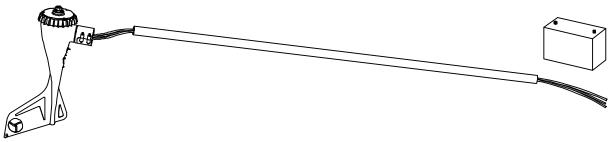
**5**/ Slide the yaw shaft all the way down over the end of pole being careful not to pinch the yaw wires. Be sure to leave enough slack in the wires so that if necessary, the Wind Generator can be removed.
