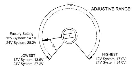
The stop charging point's factory setting is marked on the casting with a small indentation aligned with the screw slot. From the factory setting, rotate the adjusting screw 40 degree for each 0.48 (0.97) volt change desired. For example, if you want to set your voltage regulator to 14.6 (29.2) volts, turn the adjusting screw clockwise by 40 degree.
