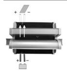
Open the cover at the battery side. Connect the wires leading to the battery with the correct polarity. To avoid any voltage from the wires, first connect the MPPT and then the wire length (min 30cm to max approx. 100cm) and the wire size: 10 mm² to 16 mm²: max. 1 m 25 mm² to 35 mm²: max. 2 m Close the cover of the battery side.
